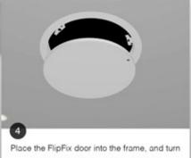
it clockwise until it locks into place. Lock the door using the plastic key supplied.
