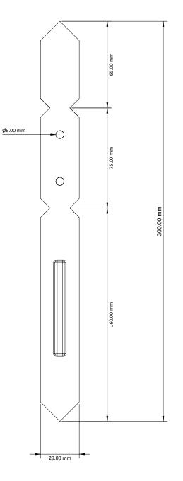
1.2mm Thick Grade of Steel = 9mm
