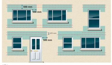
1 block course above lintel and below sill, with an additional chord 1 block apart. Extend the reinforcement a min of 500 mm past opening or where openings are closer together, create a continuous chord.
