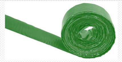
**TENMAT**'s Ventilated Fire Stop is a low profile intumescent designed for Timber and Masonry cavities. The product maintains the ventilated cavity to prevent thermal and moisture bridging and resultant damp problems, but in the event of a fire it expands to fill the cavity and prevent the spread of fire and smoke.
