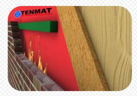
In a fire situation, the Ventilated Fire Stop will expand across the cavity to restrict the spread of fire & smoke in the cavity If the **TENMAT** Ventilated Fire Stop is cut, then the polythene sleeve should be folded around the exposed end to maintain weather protection. This should then be stapled to the sheathing board.
