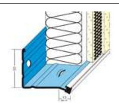
Install full system stop beads to terminate the system around the sides of the existing gas boxes and other similar features. Full System Stop beads should be 10mm wider than the board thickness for Sil TC thin coat systems.
