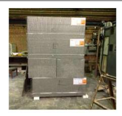
K5 phenolic foam Insulation – supplied by Kingspan pre-cut to 1.2m 0.6m size. Boards are shrunk wrapped. No of boards per pallet varies depending on the product thickness.
