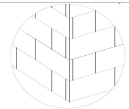
All Insulation boards should be staggered In a L Shape around window & door stress areas. Drill holes through the insulation board ensuring that the holes are drilled to the required depth in the existing wall. If the wall has existing render or dubbing out render has been applied to improve the alignment. Then the Ewi fixing length and the depth of embedment may have to be increased. The minimum embedment specified is into the main solid wall ignoring the render.
