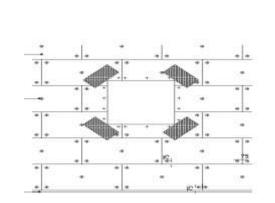
Insulation boards are interlocked at all external & internal corners & installed using a stretcher bond method. The smallest board off cut should be no less than 200mm wide x 600mm high.
